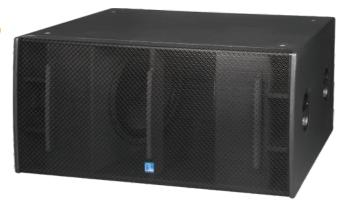
DLA218B is a dual 18" subwoofer. It features 2x18" 100mm voice coil woofer, bass-reflex design, can be used with line array and point source full range speakers to improve the low frequency performance. The cabinet is made of multilayer composite plywood with wear-resistant polyurea paint.
